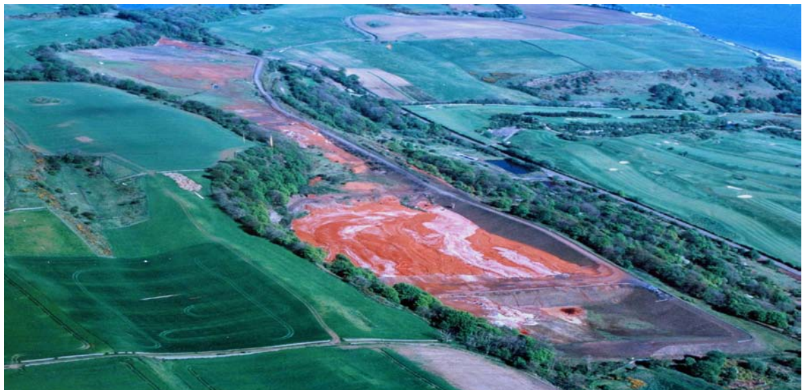
Figure 2 – Bauxite residue disposal into a former oil shale mine
